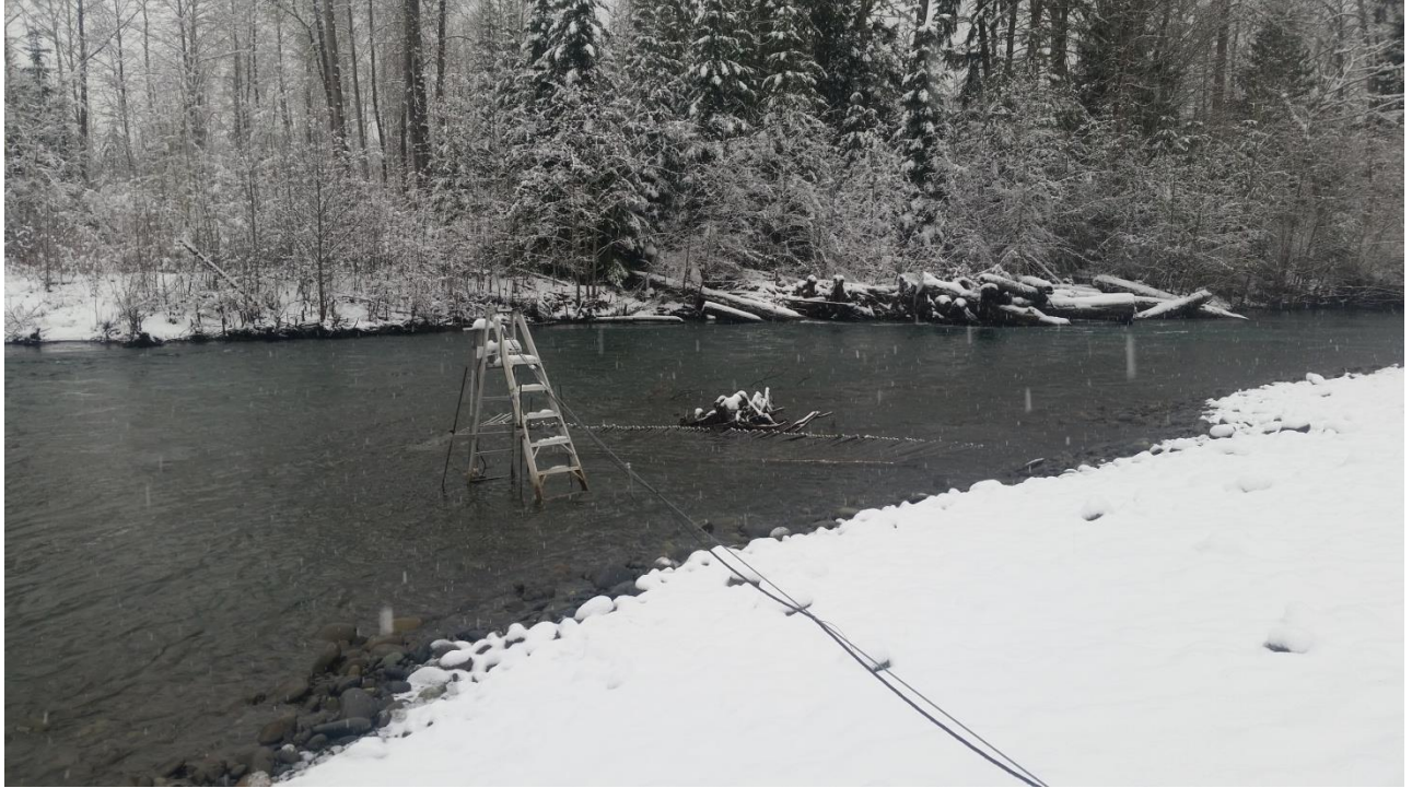
Figure 4. Old Mainstem SONAR site. The SONAR itself is attached to the pole mount which is in turn attached to the ladder. The PVC picket weir immediately downstream from the ladder directs fish away from the bank so they pass at least 3 m from the SONAR head.
